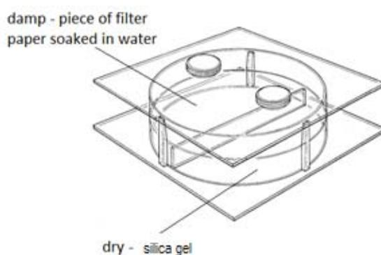
The choice chamber has been left to equilibrate (to allow conditions to become stable) before introducing the woodlice. The woodlice were introduced through the hole in the centre of the lid or cover, in a way that did not favour either end of the condition gradient.
